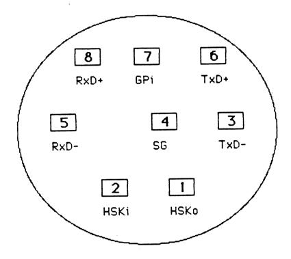
Both Serial Port 1 and Serial Port 2 have the same pin out
