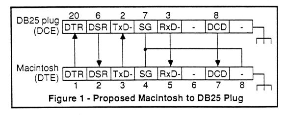
An optional cable for general purpose use is shown in figure 1a. This cable would function as a "null modem" cable and allow DTE-DTE type connections. This would also be used primarily for connecting the Macintosh to printers, some modems, etc. This cable would have an 8 pin mini-DIN plug ("male") on one end and a DB-25 plug ("male") on the other. Pin 8 on the Macintosh socket must be connected to SG, this can be done with a second wire to pin 7 of the DB25 plug.
